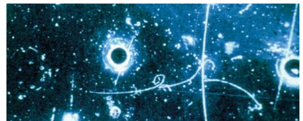
Fig. 1. A hadronic neutral current event, where the interaction of the neutrino from the left produces three secondary particles, all clearly identifiable as hadrons, as they interact with other nuclei in the liquid. There is no charged lepton.
