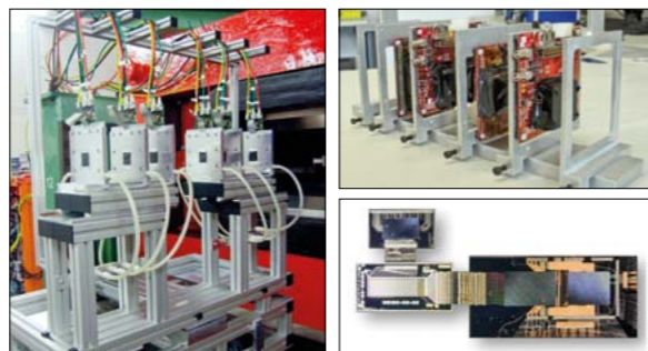
Fig. 2. Clockwise from left: Components of the combined beam-telescope in the test beam at DESY: the MIMOSA telescope, the ATLAS-FE14 arm and the DEPFET device under test. (Image credit: DESY.)
